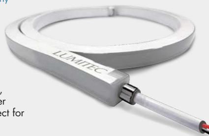
The Moray Flex Light is the only RGBW flex light in the world to have both an internal driver and an internal color/output controller. This means that Moray can be connected directly to a 2-wire DC electrical system, allowing color and dimming control with any standard on/off switch and with no external driver.
